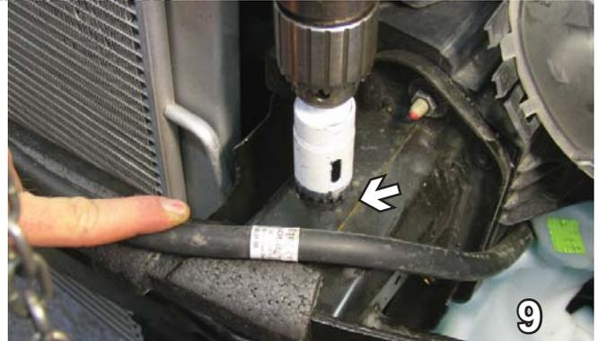
9. Remove the hose bracket and use the hole as the location to drill a hole with the 1 1/4" hole saw to use for inserting nut plates. Do this on both sides. The hose will not be replaced as it will be mounted on top of the fascia.
