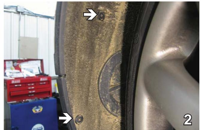
2. Forward the front tire, use a Phillips screw driver to remove two push pins. Do this to both sides and set aside for later reinstallation.
