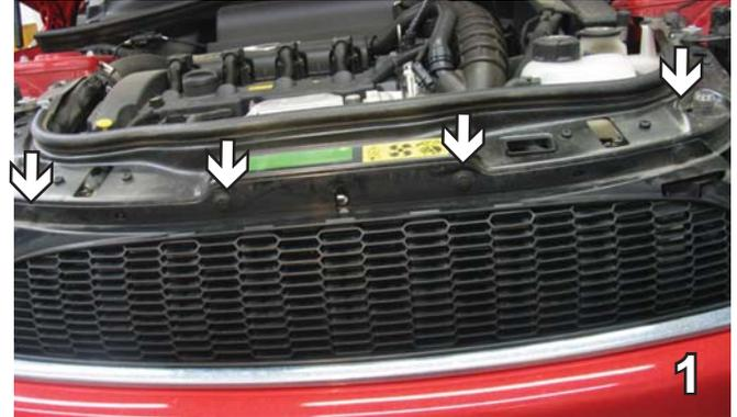
1. Using a flat screw driver, remove four push pins on top edge of grille. Set push pins aside to be reinstalled later.
