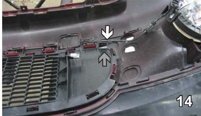
14. On the back side of the fascia, passenger side, pull up the sensor. Using a utility knife, cut off the tab (gray arrow).
