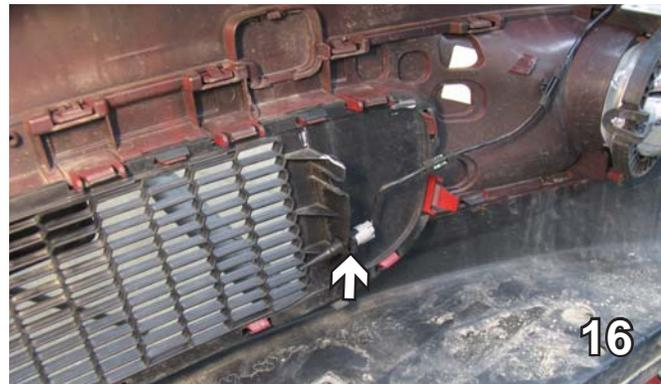
16. Make a notch and move the sensor down.
