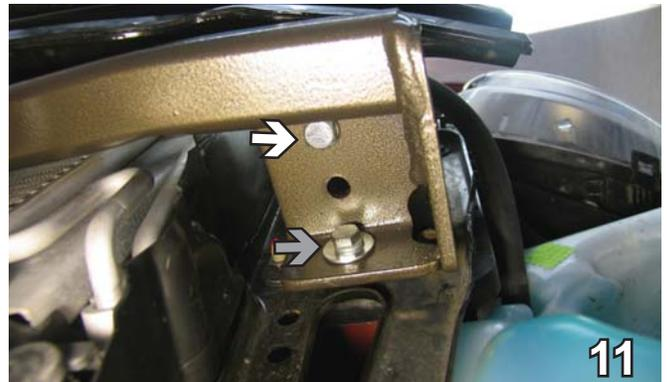
11. Insert and tighten with Loctite 3/8-16 x 1 1/4" bolt with 3/8" lock washer in the top hole and 3/8-16 nut plate inserted into the 1 1/4" hole. Then tighten with Loctite the bolt inserted in step 10 (gray arrow). Finally insert the third bolt. They must be done in this order for them all to go in.
