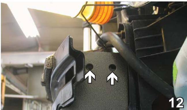
12. Using the baseplate as a template, drill the two holes on the side with a 13/32" drill bit. Insert bolts with Loctite, lock washers and nut plates.
