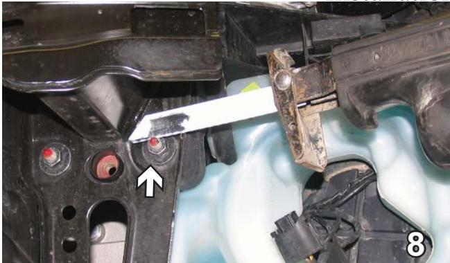
8. Use the reciprocating saw to cut off the bolt even with the nut. Do this on both sides.
