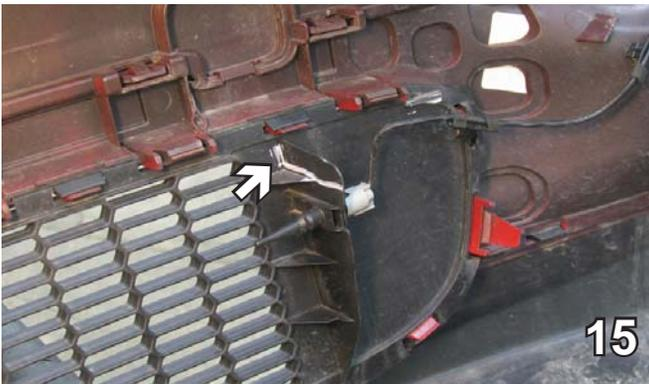
15. Continuing on the back side of the fascia, using a utility knife trim down to the gusset and straight out (as shown). Do this on both sides.
