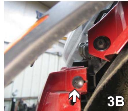
3. After removing the wheel well cover, use a flat screw driver to remove the two push pins connecting the fascia. Do this to both sides. Set push pins aside for later reinstallation. Push and release the two clips holding the gray cover, then use the T25 Torx to loosen the bolt.
