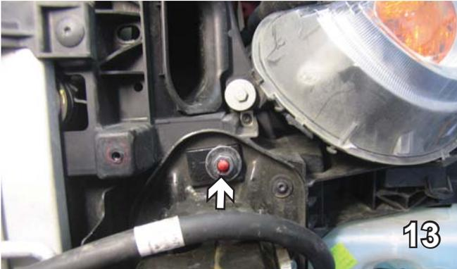
13. On top of the bumper, remove the nut add a backing plate and reinstall with Loctite. Do this on both sides.
