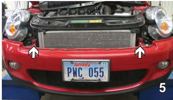
4. Remove the grille by releasing the clips. Reach in from the top and squeeze the clip together. Set aside for later reinstallation.
